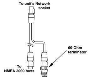
LGC-2000 Y-adapter extension cable with 60-Ohm terminator.
